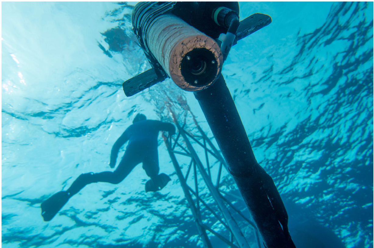
The BOUSSOLE buoy hyperspectral radiometer measuring Lu at 4 m depth, during the diving operations.
